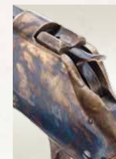
The 1885 High-Wall's loading lever (left), opens or locks the rifle's falling-block action (right).
