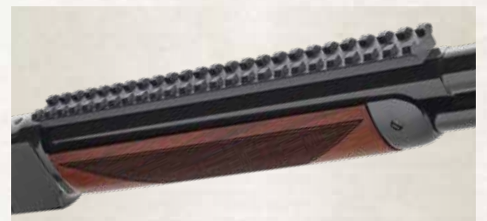
For hunters preferring optical sights, the 1873 Hunter Rifle comes with a Picatinny rail included in the box. This can be easily mounted by tapping out the buckhorn sight and screwing it on the tapped octagonal part of the barrel (all hardware included).
